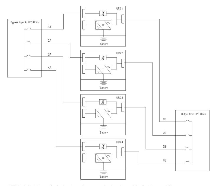
**NOTE** Required parallel system wiring length must be equal to ensure approximately equal current sharing when in Bypass mode. For proper operation the following must be true:
